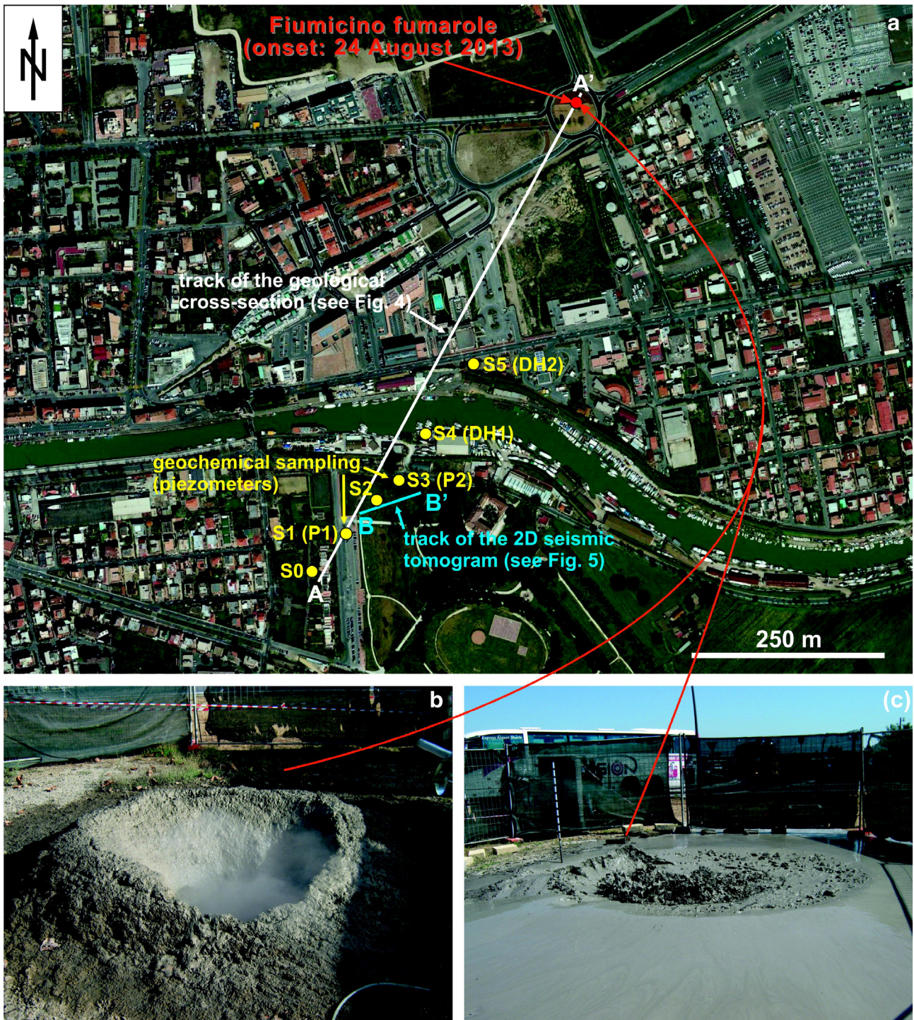
Fig. 2. (a) Location map (from Bing Maps) showing: (red) the Fiumicino fumarole (Latitude: 41^{\circ}46'32.43''\text{N} ; Longitude: 12^{\circ}14'26.57''\text{E} ); (yellow) the stratigraphic boreholes studied in this paper (Figs. 3 and 4); (white) the track of the geological cross-section shown in Fig. 4; (blue) the track of the 2D seismic tomogram shown in Fig. 5; and (yellow) the geochemical sampling sites (see related results in Figs. 6–8). The location of the water sample FI is shown in Fig. 1(b) (Table 1). (b) Photograph of the Fiumicino fumarole at the onset of its activity with the emission of mostly gases. (c) Photograph of the Fiumicino fumarole during its successive activity with the emission of gases, mud, and water. (For interpretation of the references to color in this figure, the reader is referred to the web version of this article.)
